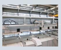
A robust torsion bar and precision rack guaranties a perfect parallelism of the pressure beam with respect to the working table. The handling of the machine becomes with a very easy and friendly control system that allows the fast implementation of cutting programs.
