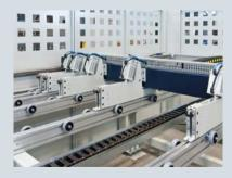
The pusher travels through precision pinions and racks. The precise positioning of the pusher is achieved by a magnetic band (no contact system). The grooved pressure beam allows the grippers to keep the panel's clamped until the final cut. The extremely fast servo-drive technology guarantees shortest cycle times.
