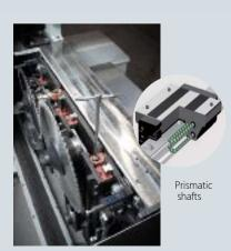
Saw blade adjustment by mechanical indicators.
