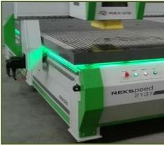
The three different color of led surrouding machine body and its changing color according to machine status. Green: Machine is Working, Yellow: Waiting command., Red: in Error
